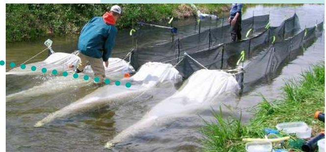
Example of **fyke nets** set-up in a part of the river to catch larval fish. Not the long-sock like fine net that funnels the small fish to the bottom where they are caught in the container.
