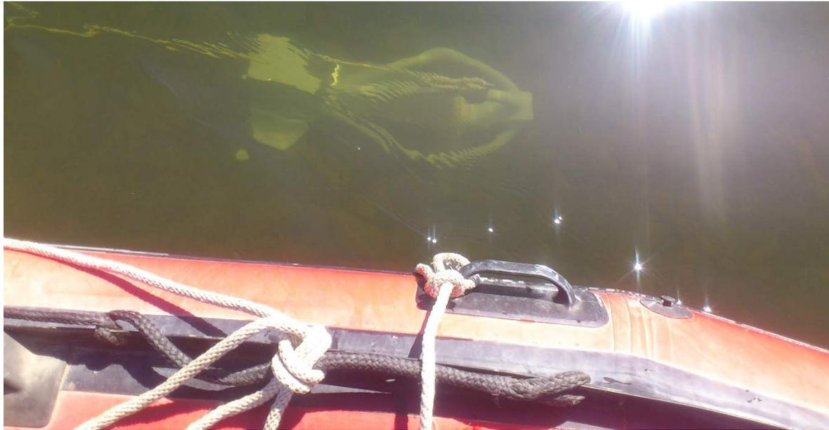
**Figure 2 Helley-Smith sampler collecting a bedload sample in 2015.**
