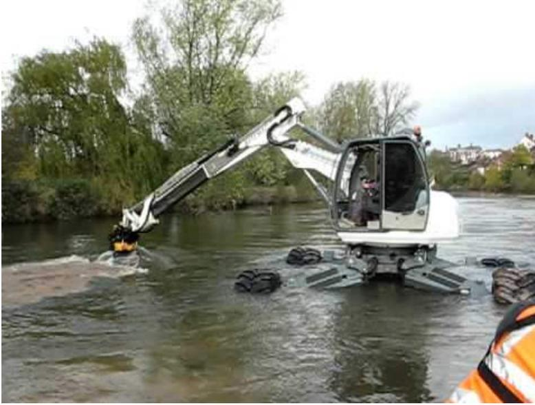
**Figure 23** Example of a walking excavator used for in-channel site restoration.
