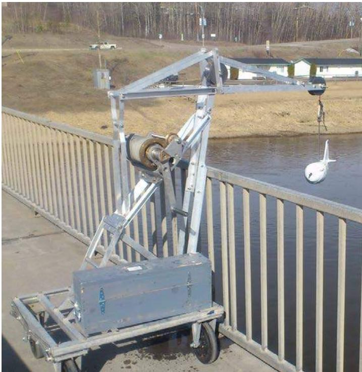
**Figure 3** Suspended sediment sampler and bridge crane.
