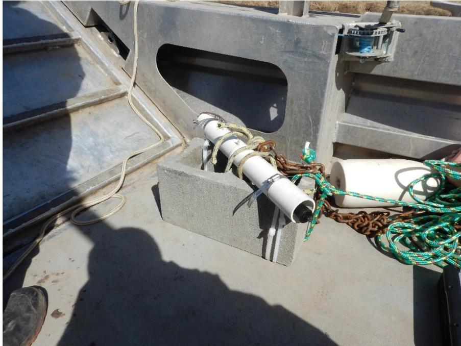
**Figure 5 Standalone turbidity sensor installed downstream of the remedial work.**
