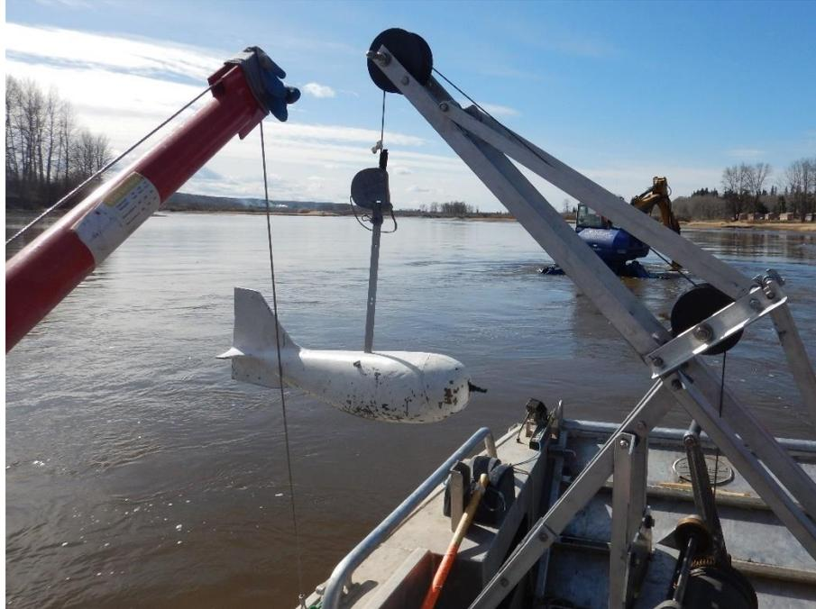
**Figure 6** Sampling suspended sediment with the D-74 sampler downstream of the excavator.
