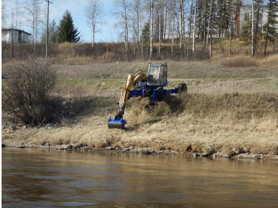
**Figure 2** S2-3 Kaiser 4x4 Spyder Walking Excavator accessing the Lower Patch directly from the north bank.
