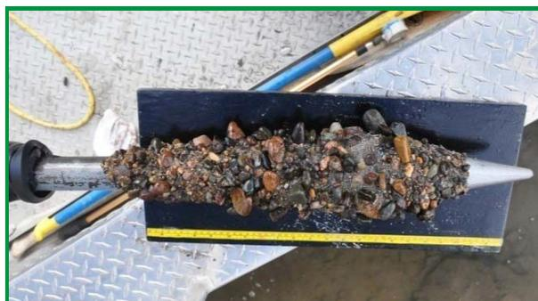
The substrate of the Upper Site is pictured on the left. The freeze core is one method used to obtain a sample of the substrate. The freeze core sample on the right was taken from the Upper Site, 2012. Photos by NHC.
