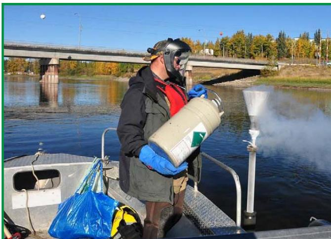
Liquid nitrogen is being poured into a funnel that has an outlet 10–30 cm above the bottom of the core, 2012. Photo by NHC and can be found in their 2012 report.
