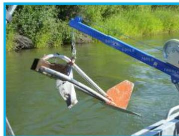
A Helley-Smith sampler was used to measure bedload. The bag collects the sediment sample.
