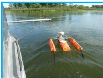
Acoustic Doppler Current Profiler was used to measure water current velocities.
